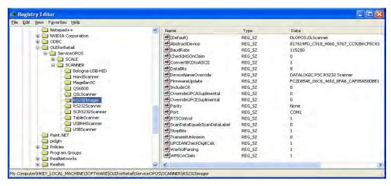
The RS232Imager utilizes a 115,200 baud rate and enhanced parsing capabilities. These registry items are turned on for this scanner type.
