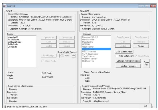
6. Click the "DataEventEnable" button and check the "AutoDataEventEnable" box, and scan a bar code. The bar code data and type will be displayed as shown here:
